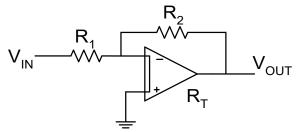
**Problem 4** Assume the amplifier shown below is designed in a 0.18 $\mu$  CMOS process with model parameters uC<sub>OX</sub>=250 $\mu$ AV<sup>-2</sup>,  $\lambda$ =0.01V, and V<sub>THn</sub>=0.4V. Assume V<sub>DD</sub>=1V, V<sub>SS</sub>=-1V, and I<sub>DQ</sub>=4mA.
