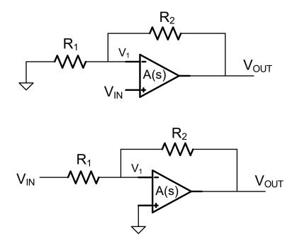
**Problem 10** (Extra Credit) The "dead network" of a circuit is obtained by setting all small-signal inputs to 0. That is, by replacing all ac voltage sources with short circuits and all ac current sources with open circuits. The  $\beta$  of a feedback amplifier is a characteristic of the "dead network". Consider the basic inverting and noninverting feedback amplifiers shown below. These are widely used as small-signal voltage amplifiers.
